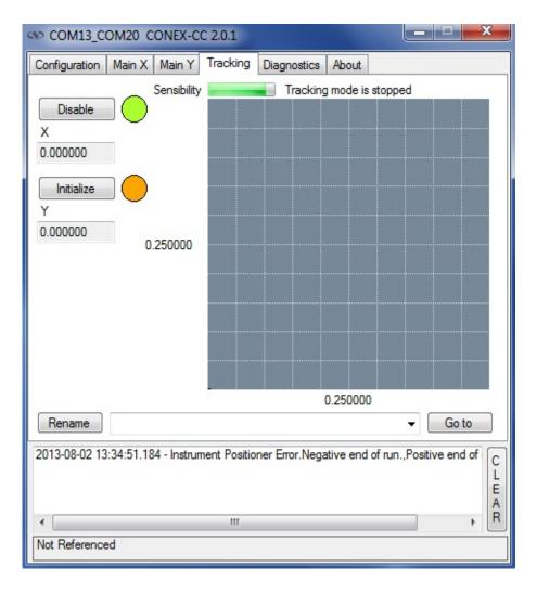
The "Enable/Disable" button executes the next enable command to change the controller status. Its name changes in relation to the controller state. To see the different controller states, refer to the controller state diagram in section 1.3.
