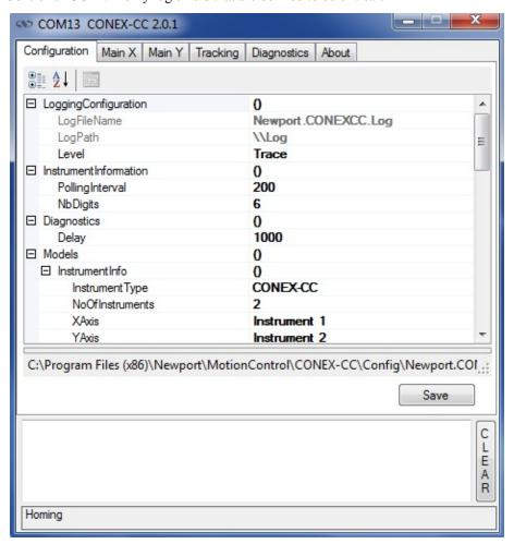
The polling interval defines the number of milliseconds between each time the Controller GUI polls the CONEX-CC for the latest information. The user may change the polling interval by entering a value. Diagnostics Delay defines the time delay in milliseconds between each command sent from a text file.
